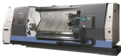
Doosan Puma 800XLM Horizontal Turning Centre Extra-large heavy duty turning centre with 5m turning capacity
